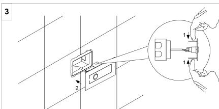
Connect the LED button cable ( 5 mt. ) To the corresponding cable present in the "F" transformer installed in zone 3
