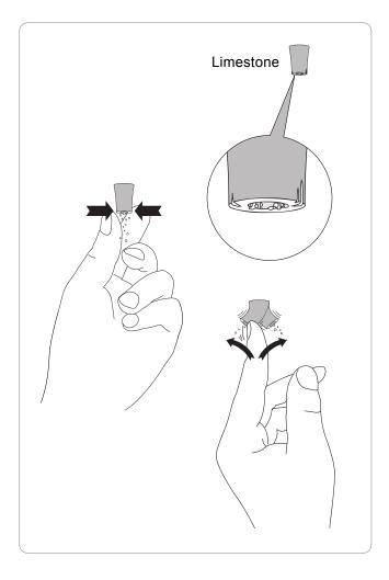
Periodically clean the nozzles to remove any lime scale as shown in Illustration.
