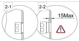
Apply the plate and make sure the junction box is alined with the plate (Fig. 2-1) or at a maximum of 15 mm. (Fig. 2-2)
