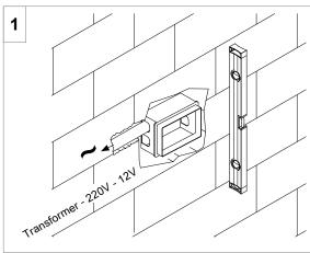
Insert the supplied junction box in the wall with the help of a level and position it properly
